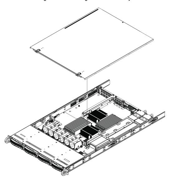
Figure 2-4. Accessing the Inside of the System
